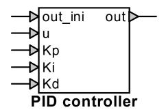
Control function: PID controller, dynamic coefficients
