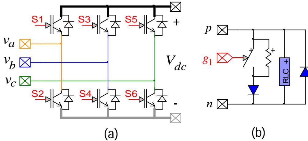
Figure 4 (a) Two-level Converter, (b) IGBT valve.
