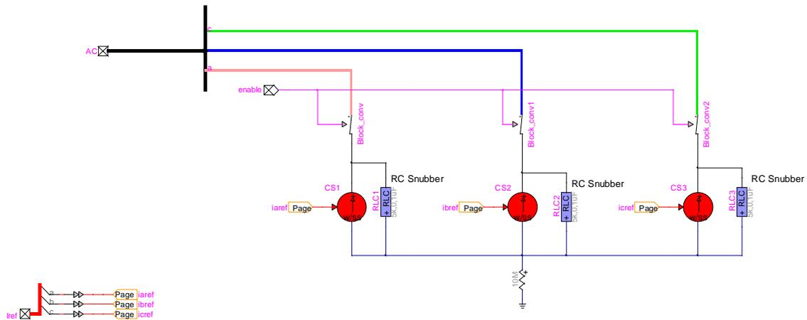
Figure 7 Current source model to support REGC\_A model.
