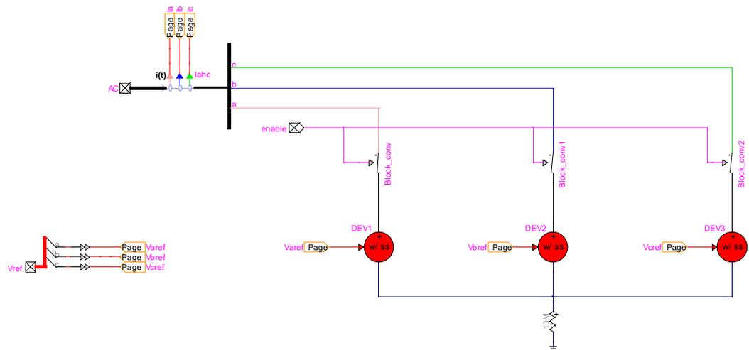
Figure 8 Voltage source model to support REGC\_C model.
