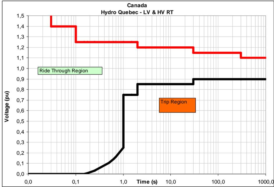
**Figure 20** LVRT and HVRT requirements [10].
