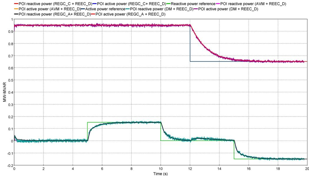
Figure 27 Active and reactive power control test.
