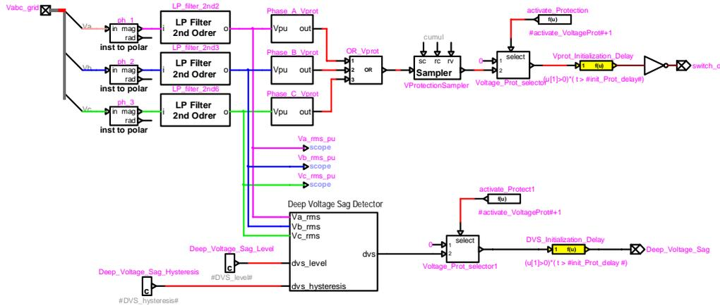
Figure 22 Over/under-voltage protections and deep voltage sag protections.
