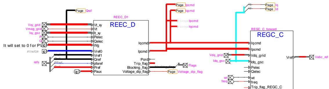
Figure 18 EMTD diagram of “control” block for REEC\_D+REGC\_C model.
