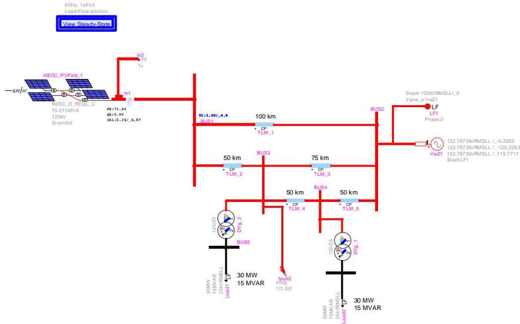
Figure 26 EPRI aggregated PV park network.
