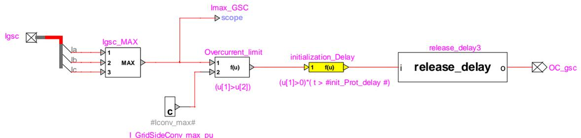
Figure 24 Overcurrent protection block.
