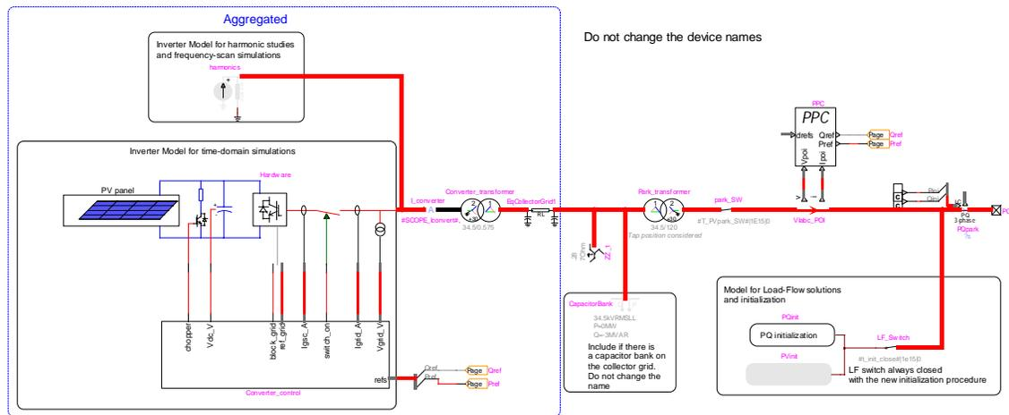
Figure 1 General structure of WECC PV park model
