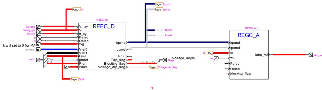
**Figure 15** EMTP diagram of “control” block for REEC\_D+REGC\_A model.
