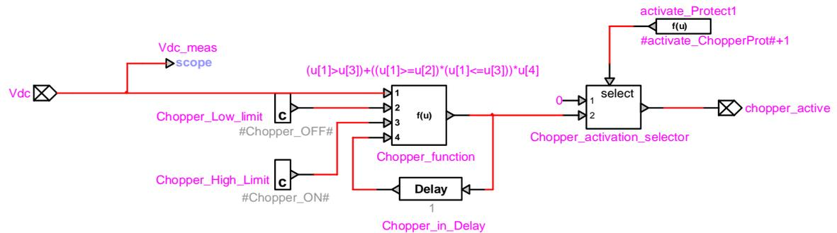
Figure 23 dc overvoltage protection block.
