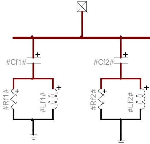
Figure 9 “shunt ac harmonic filter” block.
