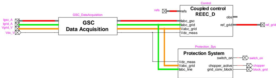
Figure 10 EMTP diagram of the PV inverter control block.
