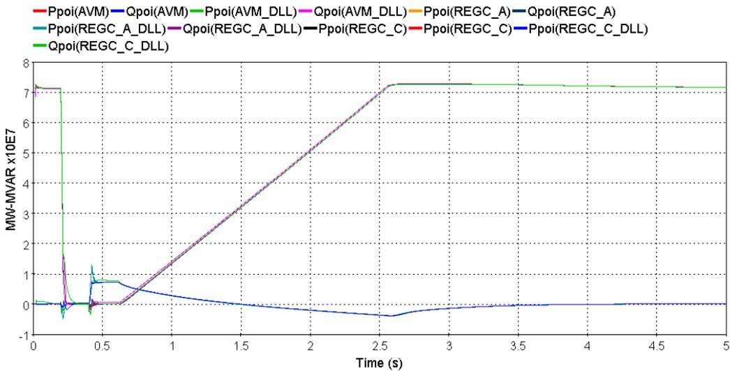
**Figure 29** Fault test: POI active power, POI reactive power.
