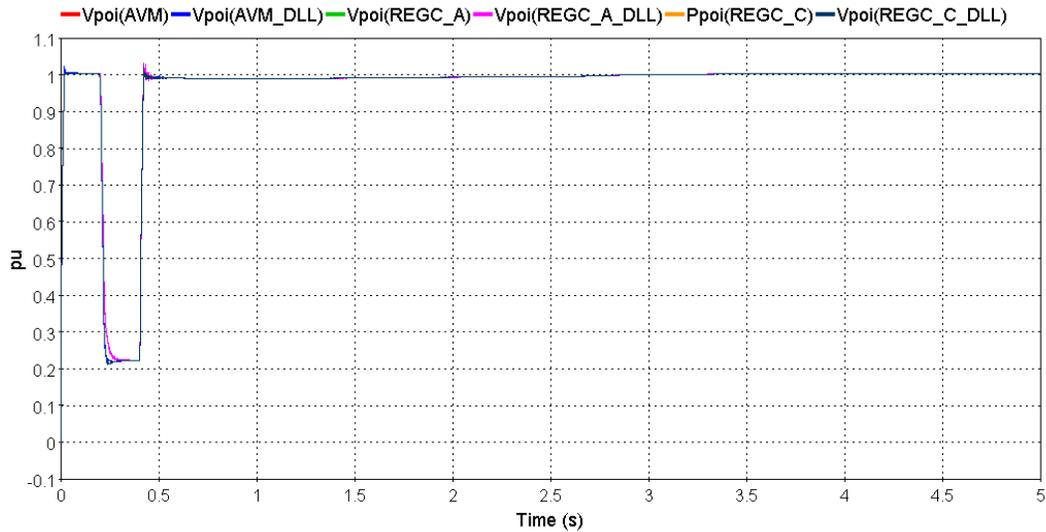
**Figure 28** LVRT test: RMS voltage at POI.
