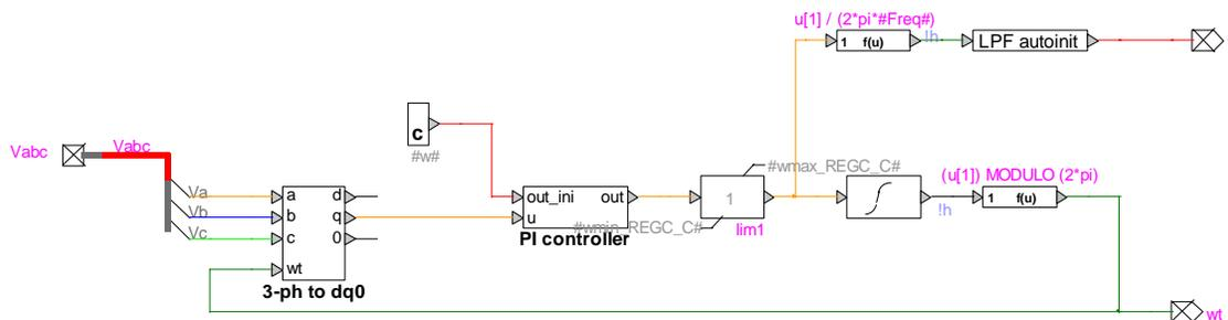
Figure 17 PLL model used in REGC\_A + REEC\_D model.
