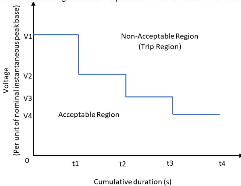
**Figure 21** Transient overvoltage limits.
