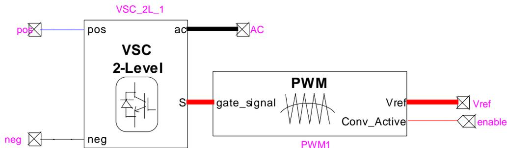
Figure 3 DC-AC converter block inside the inverter hardware model (detailed model version).
